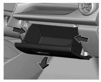
1. Open the glove box door completely.
