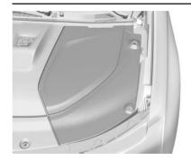
The emergency manual charge cord release is below the underhood access covers. To remove, see *Underhood Access* Covers
