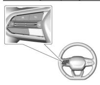
: Press to turn the system on or off. The ACC indicator light — displays white on the instrument cluster when ACC is turned on.
