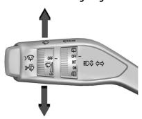
Move the lever all the way up or down to signal a turn.
