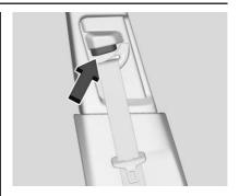
Press the release button and move the height adjuster to the desired position. The adjuster can be moved up by pushing the slide/trim up. After the adjuster is set to the desired position, try to move it down without pressing the release button to make sure it has locked into position.
