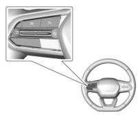
᠍ : Press to turn cruise control on or off. The cruise control indicator appears white when cruise control is turned on. See *Cruise Control Light* ⇒ 99
