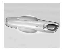
Insert the cap back into the grooves on the door handle.
