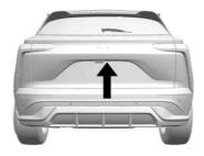
To open the liftgate, press on the power door lock switch or press on the remote key twice to unlock all doors. Press the touchpad on the underside of the liftgate handle and lift up.
