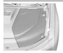
2. The underhood compartment fuse block is below the underhood access covers. To remove, see *Underhood Access Covers* ⇒ 265.
