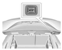
• Press 22 on the buttom of the liftgate next to the pull cup to close.
