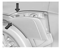
Push the top left corner of the charge port door and release to open the door.
