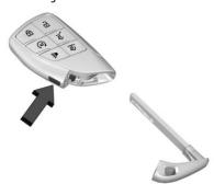
To remove the mechanical key, press the button near the bottom of the remote key, and pull the key out. Never pull the mechanical key out without pressing the button.
