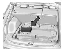
Release the strap securing the tire sealant and compressor kit, then remove the kit.
