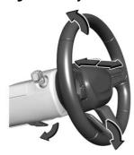
To adjust the steering wheel, if equipped:
