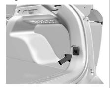
The vehicle has two cargo tie-downs in the rear compartment. Open the cover to access.
