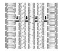
Treadwear indicators are one way to tell when it is time for new tires. Treadwear indicators appear when the tires have only 1.6 mm (1/16 in) or less of tread remaining. See *Tire Inspection* ⇒ 296 and *Tire Rotation* ⇒ 296.
