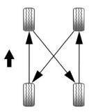
Use this rotation pattern if the vehicle is equipped with rear wheel drive.
