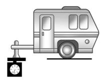
The trailer tongue weight contributes to the Gross Vehicle Weight (GVW). GVW includes the CURB WEIGHT of your vehicle, any passengers, cargo, equipment and the trailer tongue weight. Vehicle options, passengers, cargo, and equipment reduce the maximum
