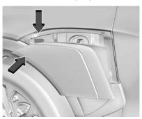
Push the top left corner of the charge port door and release to open the door. In cold weather conditions, ice may form around the charge port door. Remove ice from the area before attempting to open or close the charge port door.
