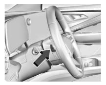
Regen on Demand allows for increased deceleration by pressing and holding the steering wheel paddle. Regen on Demand works in D (Drive). The accelerator pedal can be used to manage deceleration while using Regen on Demand. See *One-Pedal Driving* \$\pi\$ 174.
