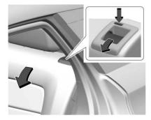
Pull the handle on top of the seatback to unlock it.
