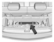
The warning triangle is stored in the rear of the vehicle under the load floor.
