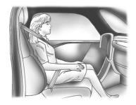
If a person of adult size is sitting in the front outboard passenger seat, but the OFF indicator is lit, it could be because that person is not sitting properly in the seat or that the child restraint locking feature is engaged. Use the following steps to allow
