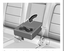
If equipped, cupholders are located in the second row seat armrest. To access, pull the armrest down. The cupholder liner is not removable.
