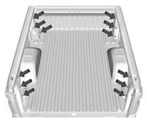
This vehicle is equipped with 12 fixed cargo tie-downs.
