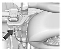
If equipped with a spare tire cable, reattach the clip to the frame attachment bracket. Note that there may be slack in the cable.
