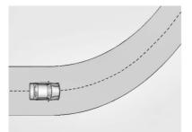
When entering a curve, Super Cruise may not detect the lane markings and may not adjust the steering enough to stay in your lane of travel. When this happens, you will need to steer the vehicle.
