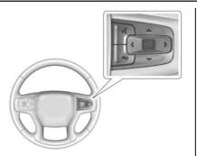
$\lhd$  or  $\triangleright$ : Press to move left or right between the interactive display zones in the instrument cluster. Press the thumbwheel to select.
