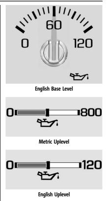
The engine oil pressure gauge shows the engine oil pressure in kPa (kilopascals) or psi (pounds per square inch) when the engine is running.
