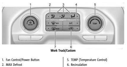
7. Rear Window Defogger (If Equipped) or Heated Mirrors (If Equipped)
