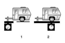
The trailer tongue weight (1) should be 10–15% and fifth-wheel or gooseneck tongue weight should be 15–25% of the total loaded trailer weight (2). Some specific trailer types, such as boat trailers, fall outside of this range. Always refer to the trailer owner's manual for the recommended trailer tongue weight for each trailer. Never exceed the maximum loads for the vehicle, hitch, and trailer.
