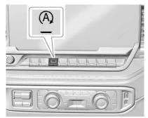
The automatic engine Stop/Start feature can be disabled and enabled by pressing  $\triangle$ . Auto Stop/Start is enabled each time you start the vehicle.
