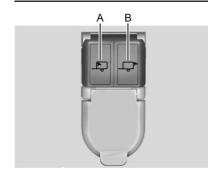
If equipped, trailering camera connectors are available in the bumper trailer receptacle in place of the four-pin connector. The inside trailer auxiliary camera should be installed on the top left hand side (A) and the rear trailer auxiliary camera (B) should be installed on the top right hand side.
