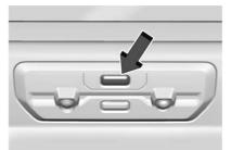
The MultiFlex inner tailgate may be equipped with an enable/disable feature to prevent the inner tailgate from being opened when a hitch or other equipment is installed that could damage the inner tailgate.
