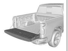
Press x twice quickly on the remote key until the tailgate moves. See *Remote Key Operation* ⇒ 12. If equipped with Keyless Access, the tailgate can be opened if the remote key is within 1 m (3 ft).
