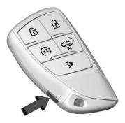
If the vehicle has the Keyless Access system, the remote key has a button on the side of the remote key used to remove the key.
