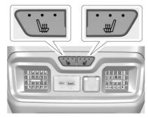
If available, the buttons are on the rear of the center console. To operate, the engine must be running.
