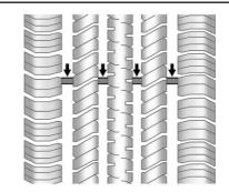
Treadwear indicators are one way to tell when it is time for new tires. Treadwear indicators appear when the tires have only 1.6 mm (1/16 in) or less of tread remaining. See *Tire Inspection*  $\Rightarrow$  390 and *Tire Rotation*  $\Rightarrow$  390.
