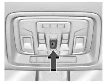
If equipped, the power sliding rear window works when the ignition has been turned on or to accessory mode, or Retained Accessory Power (RAP) must be active. See *Retained Accessory Power (RAP)*  $\Rightarrow$  219.
