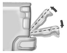
To close the tailgate using the lift-to-close feature, lift the tailgate from the full-open position to at least 10 cm (4 in) and hold it momentarily. Then, the tailgate will start closing automatically. If the tailgate is lifted more than halfway between open and close, then it will not close automatically.
