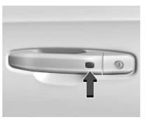
If equipped, the remote key must be within 1 m (3 ft) of the tailgate or door being opened or locked. Press the button on the door handle to open. See "Keyless Access Operation" in *Remote Key Operation*  $\Rightarrow$  12.
