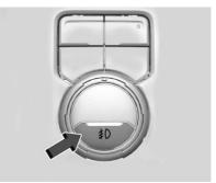
If equipped, the fog lamp control is near the exterior lamp control to the left of the steering column.
