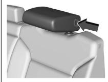
The head restraint can be folded forward to allow for better visibility when the rear seat is unoccupied. To fold the head restraint, press the button on the side of the head restraint.
