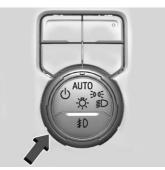
The exterior lamp controls are on the instrument panel to the left of the steering wheel.
