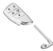
Press the button to remove the key. Never pull the key out without pressing the button.
