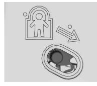
The safety lock is on the inside edge of the rear doors. To use the safety lock:
