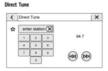
Access Direct Tune by touching the Tune icon on the AM, FM, or SiriusXM screen to bring up the keypad. Navigate up and down through all frequencies using  $\mathbb{K} \$  or  $\mathbb{N}$ . Directly enter a station or channel using the keypad. When a new station or channel is entered, the information about that station or channel displays on the right side. This information updates with each new valid frequency tuned to.
