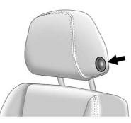
To raise or lower the head restraint, press the button on the side of the head restraint and pull up or push the head restraint down and release the button.
