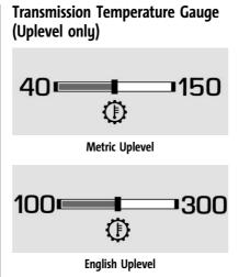
This gauge displays while the vehicle is in the Tow/Haul driver mode, and the lower gauges are configured to display four gauges. The transmission fluid temperature is also selectable as Left/Right side info. To change gauge configurations, see "Options" under *Instrument Cluster (Base Level)*  $\Leftrightarrow$  108 or
