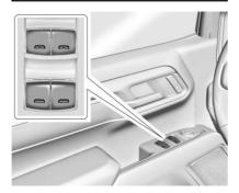
The power windows work when the vehicle is on, in accessory mode, or when Retained Accessory Power (RAP) is active. See Retained Accessory Power (RAP) ⇔ 219. Using the window switch, press to open or pull to close the window.
