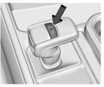
${\bf P}$  : This position locks the rear wheels. Use P (Park) when starting the engine to prevent the vehicle from moving easily.
