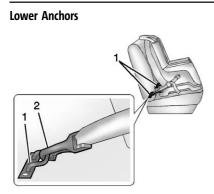
Lower anchors (1) are metal bars built into the vehicle. There are two lower anchors for each LATCH seating position that will accommodate a child restraint with lower attachments (2).
