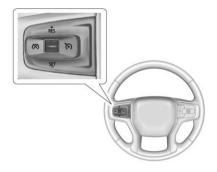
ress to turn cruise control on or off. The cruise control indicator light is lit white on the instrument cluster when cruise control is turned on
