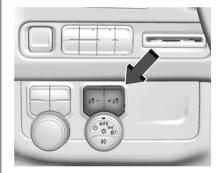
This feature adjusts the brightness of all illuminated controls. The instrument panel illumination control is above the exterior lamp control.
