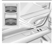
The power windows work when the vehicle is on, in accessory mode, or when Retained Accessory Power (RAP) is active. See Retained Accessory Power (RAP) ⇔ 219.
