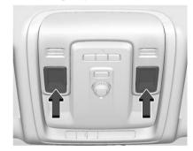
The front reading lamps are in the overhead console. Press the lamp lenses to turn the front reading lamps on or off.
