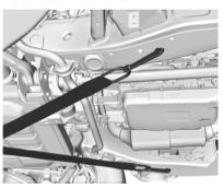
The vehicle is equipped with specific attachment points to be used to pull the vehicle onto a flatbed car carrier from a flat road surface. Do not use these attachment points to pull the vehicle from snow, mud or sand.
