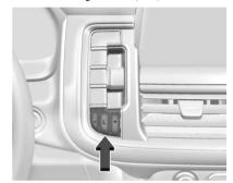
ERS or manual mode allows for the selection of the range of gear positions. Use this mode when driving downhill or towing a trailer to limit the top gear and vehicle speed. The shift position indicator within the Driver Information Center (DIC) will display a number next to the L indicating the highest available gear under manual mode and the driving conditions when manual mode was selected.
