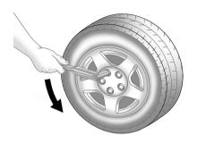
Use the wheel wrench to loosen all the wheel nuts. Turn the wheel wrench counterclockwise to loosen the wheel nuts. Do not remove the wheel nuts yet.
