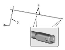
2. Assemble the jack handle extensions (4) and wheel wrench (5), as shown.
