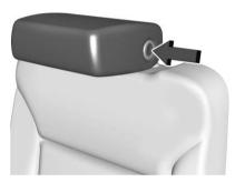
The head restraint will fold forward automatically.
