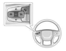
Press to turn cruise control on or off. When ACC is the selected cruise control mode, the ACC indicator light, of or , is lit white on the instrument cluster.
