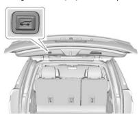
Press on the bottom edge of the liftgate next to the latch to close. Press any liftgate button, the touch pad, or on the remote key while the liftgate is moving to stop it. Pressing any liftgate button or pressing with twice quickly on the remote key restarts the operation in the reverse direction. Pressing the touch pad on the liftgate handle will restart the motion, but only in the opening direction.
