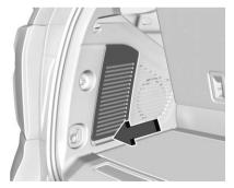
The rear compartment fuse block is behind the access panel on the left side of the compartment.
