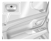
The indicator light, on the driver door near the window, indicates the status of the system. See *Power Door Locks* ❖ 16
