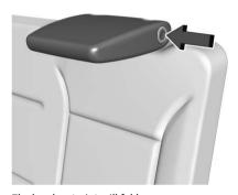
The head restraint will fold forward automatically.
