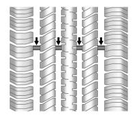
Treadwear indicators are one way to tell when it is time for new tires. Treadwear indicators appear when the tires have only 1.6 mm (1/16 in) or less of tread remaining. See *Tire Inspection* ♀ 377 and *Tire Rotation* ♀ 377.
