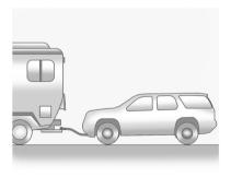
Only dinghy tow four-wheel-drive vehicles with a two speed transfer case that has an N (Neutral) and a 44 setting.
