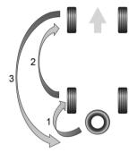
Remove the rear tire and replace it with the spare tire by performing all steps in Removing the Flat Tire and Installing the Spare Tire.
