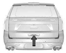
To open the liftgate, press on the power door lock switch or press on the remote key twice to unlock all doors. Press the touch pad (1) on the underside of the liftgate handle and lift up.
