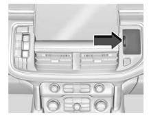
There is storage on the instrument panel. To open, if the storage is covered, press the button and slide the cover until it locks.
