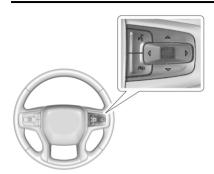
**or or :** Press to move left or right between the interactive display zones in the instrument cluster. Press the thumbwheel to select.
