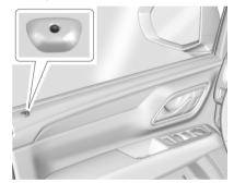
A light on the upper surface of the driver door trim is used to indicate vehicle security status.
