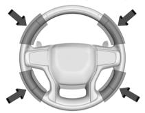
To begin steering manually, hold the steering wheel firmly with both hands using the highlighted regions. The Super Cruise indicator light will display red and a message will display in the DIC. In addition, beeps will sound, or the Safety Alert Seat will vibrate, if equipped. To view collision and detection settings from the infotainment home screen, touch Settings > Vehicle > Collision/Detection Systems. When you begin steering manually, Super Cruise will disengage.
