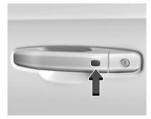
The remote key must be within 1 m (3 ft) of the liftgate or door being opened or locked. Press the button on the door handle to open. See "Keyless Access Operation" in Remote Key Operation ♀ 8.
