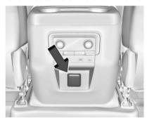
When the ignition is on, power to the 110 Volt outlet is enabled. 110 Volt power is supplied to the outlet when it is enabled and electrical equipment is plugged into that outlet. One power outlet can be used with electrical equipment that uses a maximum of 400 watts. Ensure that all connected devices do not exceed 400 watts.
