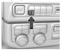
The button for TCS and StabiliTrak/ESC is on the instrument panel to the left of the steering wheel.
