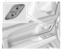
: Press to lock the doors. The indicator light in the switch will illuminate when locked.
