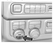
Press the Ride Height button to open the Ride Height Menu on the Instrument Panel.
