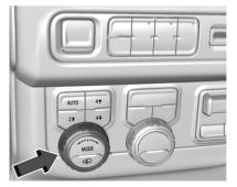
Turn the knob left or right to select the desired ride height in the menu. To finalize the selection, either press the Ride Height button again or wait three seconds for the menu to timeout. Ride Heights that are unavailable for selection will be greyed out in the menu.
