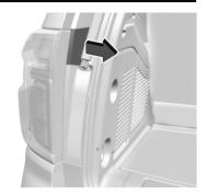
Remove the middle trim piece by pulling towards the center of the vehicle to disengage the clips.
