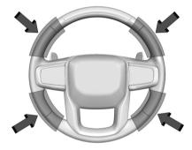
If your vehicle is equipped with Super Cruise or Lane Centering Assistance, hold the steering wheel in the indicated areas to help prevent unwanted take steering alerts.
