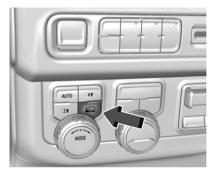
To activate Terrain Mode, press the Terrain Mode button located next to the Mode knob.
