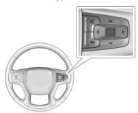
or : Press to move left or right between the interactive display zones in the instrument cluster. Press the thumbwheel to select. △ or ▽: Use the thumbwheel to scroll up or down in a list. Press the thumbwheel to open a menu or select a menu item. Press and hold to reset values on certain screens.
