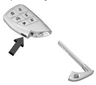
Press the button on the side of the remote key and pull the mechanical key out.
