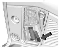
2. Turn the jack knob counterclockwise to release the jack and wheel blocks from the bracket. If equipped, remove the wheel blocks from the jack and place the wheel blocks on both sides of the tire at the opposite corner of the tire being changed. See If a Tire Goes Flat ⇒ 383 for more information on the placement of the wheel blocks. Place the jack and wheel blocks near the tire being changed.
