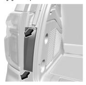
Remove the lower taillamp closeout cover from the taillamp assembly by pulling rearward from the top and bottom to disengage the clips.
