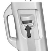
Push the release button to move the height adjuster to the desired position.
