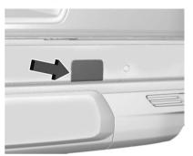
Open the spare tire lock cover on the bumper and use the mechanical key to remove the spare tire lock (6). To remove the spare tire lock, insert the mechanical key, turn, and pull straight out.
