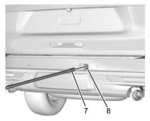
Insert the hoist end (open end) of the extension tool (7) through the hoist shaft access hole (8) in the rear bumper until you feel engagement with the hoist assembly (1). Only a minimal amount of the jack handle extension end will be visible
