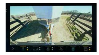
**Rear Camera View** Displays a view behind the truck with available guidelines to assist with parking and tight manoeuvres or to hitch a trailer.
