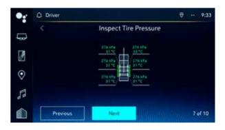
Trailer Tire Pressure and Temperature Monitoring<sup>2</sup> This available feature checks the pressure and temperature of the air inside of up to six trailer tires to help detect potential blowouts.
