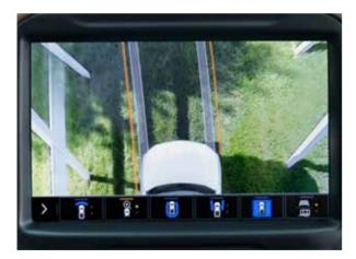
**Front Top-Down View** Provides a top-down view of the hood, bumper and front tires for tight manoeuvres in parking lots or along curbs. Includes guidelines that can be turned on or off as necessary.
