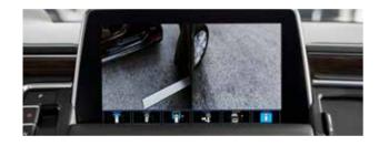
**Front Side View** Shows the position of the front tires when parking and during tight manoeuvres.
