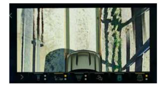
Front Top-Down View Provides a top-down view of the hood, bumper and front tires for tight manoeuvres in parking lots or along curbs. Includes guidelines that can be turned on or off as necessary.
