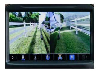
Rear Side View Provides a line of sight down each side of the truck and trailer via a split screen. This view is available while in Drive or Reverse and includes a turn signal-activated biasing view and a Trailer Length Indicator.
