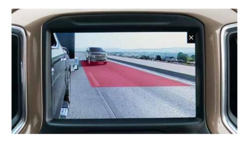
**Rear Side View (Turn Signal Activated)** With a compatible trailer attached and a turn signal activated, this view will show a full screen down the side of the truck along with a Trailer Length Indicator to aid in lane-change manoeuvres by visually showing obstructions with the trailer in adjacent lanes.
