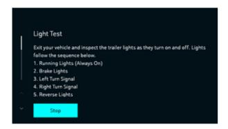
**Trailer Light Test** To help you check that all of your truck and trailer lights are in working order, this feature activates your brake lights and turn signals so you can perform a visual inspection.
