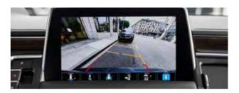
**Rear Camera View** Displays a rear view to assist with parking and tight manoeuvres.
