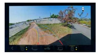
Rear Trailer View¹ Uses an available accessory camera to show objects behind a compatible trailer. Trailer Angle Indicator with Trailer Guidelines¹ shows your current path. A second set of guidelines shows where the trailer will go based on steering inputs.
