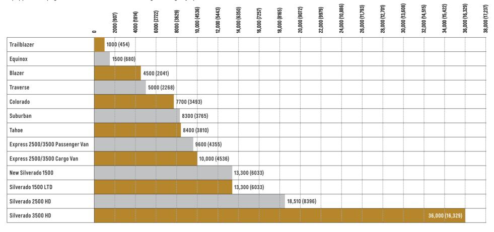
**Silverado Series** In general, a higher series number in a model indicates a greater load-carrying capacity. In addition, a truck with a higher series number typically has a stronger frame, a stiffer suspension and higher-capacity brakes, increasing the truck's ability to trailer heavy loads.
