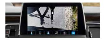
**Hitch View** Provides a close-up view of the receiver hitch to help with alignment when connecting to a trailer.
