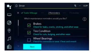
Maintenance Reminders Provides trailer maintenance reminders for things like brakes, tires and wheel bearings based on time or mileage.
