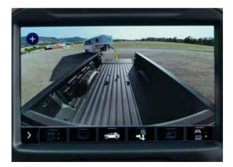
**Bed View with Guidance** Bed Hitch Guidance is now available to help align and hook up a fifth-wheel or gooseneck trailer.
