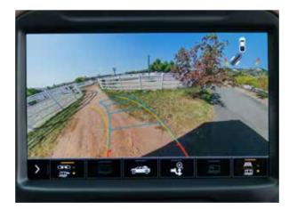
Rear Trailer View¹ Uses an available accessory camera to show objects behind a compatible trailer. Trailer Angle Indicator with Trailer Guidelines¹ shows your current path. A second set of guidelines shows where the trailer will go based on steering inputs.
