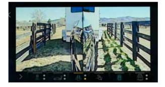
Rear Side View Provides a line of sight down each side of the truck and trailer via a split screen. This view is available while in Drive or Reverse and includes a turn signal-activated biasing view and a Trailer Length Indicator.
