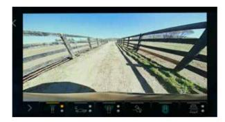
**Front Camera View** Displays a view in front of the truck with available guidelines to assist with parking and tight manoeuvres.
