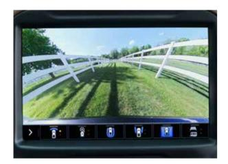
**Front Camera View** Displays a view in front of the truck with available guidelines to assist with parking and tight manoeuvres.
