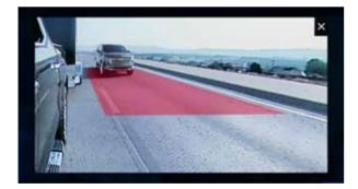
Rear Side View (Turn Signal Activated) With a compatible trailer attached and a turn signal activated, this view will show a full screen down the side of the truck along with a Trailer Length Indicator to aid in lane-change manoeuvres by visually showing obstructions with the trailer in adjacent lanes.
