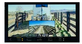
**Pic-In-Pic Side View**<sup>1</sup> Combines two views — the Rear Side View and the Rear Trailer View. Requires available Chevrolet Accessory Camera.
