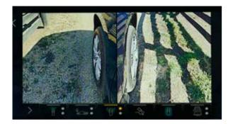
**Front Side View** Shows the position of the front tires when parking and during tight manoeuvres.
